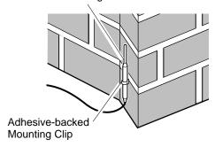
Figure 33 - Locating Thermostat Sensing Bulb on Masonry Fireplace
